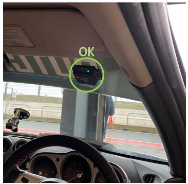
▲ **Alternative**: *Racelink* positioned on the window, below the windscreen window streamer. Do not forget to properly fit the 3M Dual Lock Velcro (or other fixing material).
